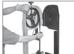
4. Loosen, but do not remove the lower hex bolt in the blade wheel tilting mechanism.
