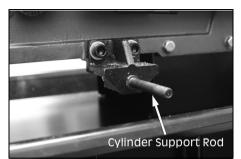
Slide the cylinder onto the rod, as shown, with the feed rate control knob pointing upwards and refit the retaining nut into position at the end of the support rod.
