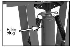
Ensure that any defective hydraulic components are replaced before using. In the event of leaking seals, oil can be topped up via the filler plug on the ram. Oil should be level with the bottom of the hole. If necessary top up with CLARKE hydraulic oil, Part No. 3050830 (1 litre). This task is carried out with the ram fully retracted.
